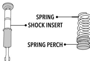
Rear divorced spring setups have the spring mounted on a separate adjustable spring perch. The ride height must be set with the rear spring and spring perch assembly before the shock can be extended so that there is no slack and the spring is preloaded exactly to the shock length.
