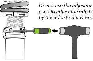
Do not use the adjustment wrench to lock the lower mount, it is only used to adjust the ride height. If the lower locking collar is tightened by the adjustment wrench, it MAY COME LOOSE.
