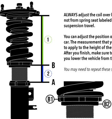
ALWAYS adjust the coil over height from the lower shock mount labeled (A), not from spring seat labeled (B). By doing this, you will not tamper with the suspension travel.
