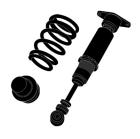
Applications with rear divorced spring setups have the spring mounted on a separate adjustable spring perch. Setting the proper spring pre-load on a divorced spring setup is achieved by setting the ride height with the rear spring and spring perch assembly first. Once the ride height is set with the spring, the shock should be extended so that there is no slack and the spring is pre-loaded exactly to the shock length.
