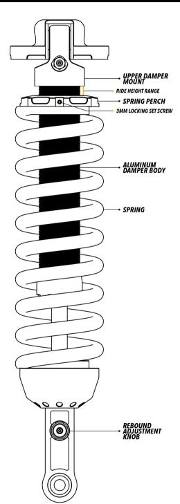
Fortune Offroad suspension uses spring perch height to determine ride height. Threading the spring perch away from the upper damper mount will raise the ride height, and threading the spring perch toward the upper damper mount will lower the ride height.
